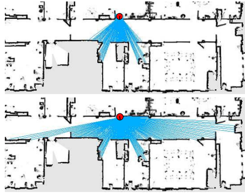
Fig. 1. In mobile robot localization, small variations in the robot pose can cause large variations of the range measurements. This leads to multi-modal distributions of beam-lengths even in small areas around a potential pose.
